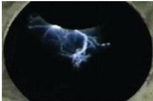
**Figure 2. Spark discharge in a hydraulic reservoir.**
